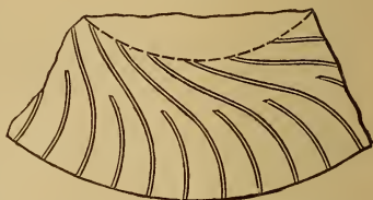
Part of the wheel, Fig. 4074, drawn on a larger scale to show the curvature of the vanes more correctly.
